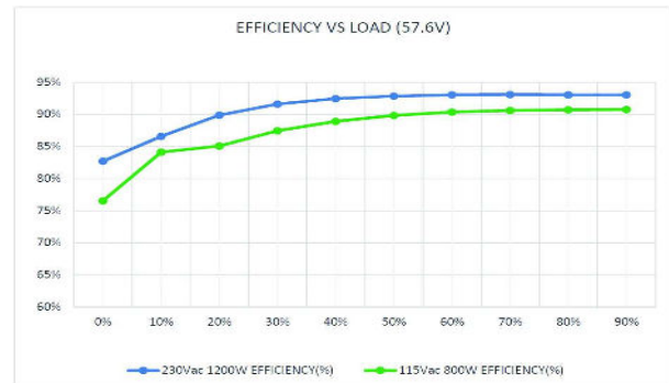
Figure 9. Efficiency Curves for LCC1200-48U with 57.6 V Output
