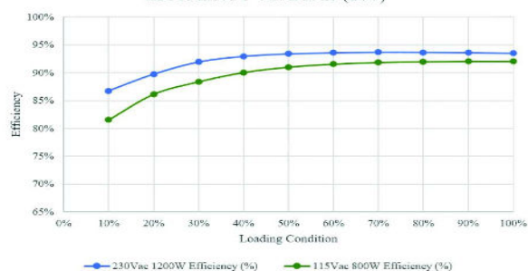
Figure 4. Efficiency Curves for LCC1200-28U with 24 V Output
