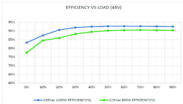
Figure 8. Efficiency Curves for LCC1200-48U with 48 V Output
