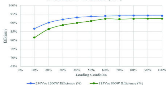
Figure 5. Efficiency Curves for LCC1200-28U with 28 V Output
