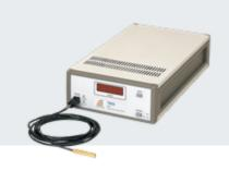
The Trek® 370 precision electrostatic voltmeter for non-contacting surface voltage measurements in the range of 0 to ±3 kV DC or peak AC. The Trek 370 employs an electrostatic field-nulling technique which achieves high DC stability and high measurement accuracy even if the probe to measured surface spacing changes. This permits measurements of either stationary or moving surfaces without the need to establish fixed spacing to maintain accuracy.
