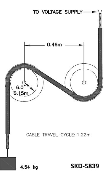
failure occur during the 77,800 cycles, the best specimen shall be removed from the test apparatus and an ac step voltage withstand test to breakdown shall be performed for engineering information only. The filament conductors shall be withstand tested for one minute at 5000v, for engineering information only.
