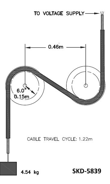
**PERFORMANCE CRITERIA:** The specimen shall maintain the test voltage for the entire flex duration without failure.
