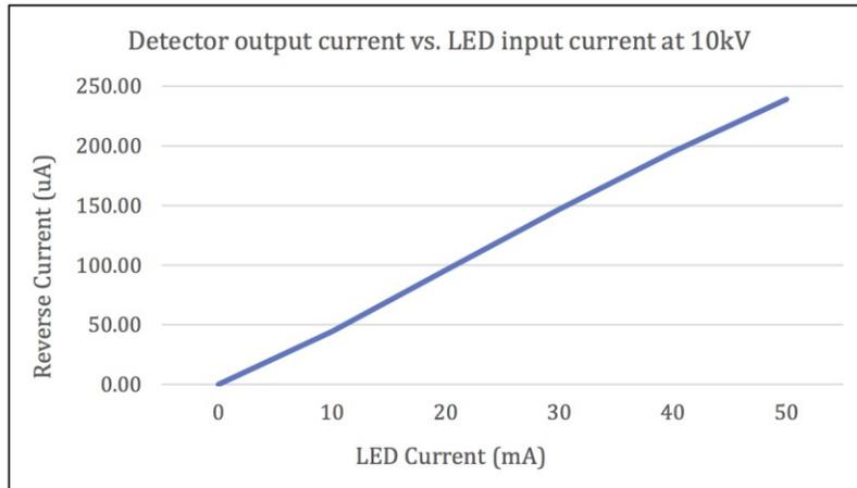
**Figure 2: Photo Detector Diode Current vs. LED Current**
