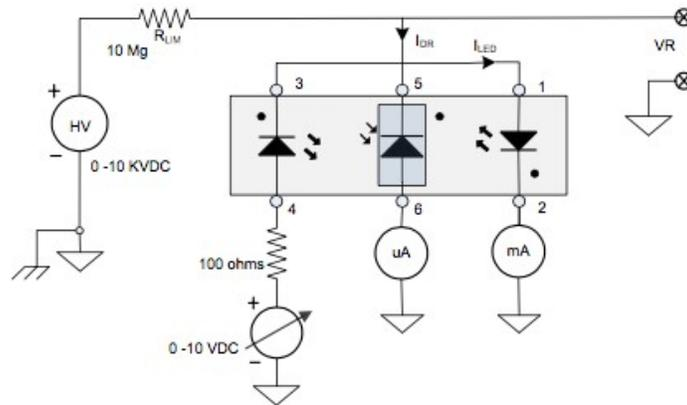
**Figure 1: Test Circuit**
