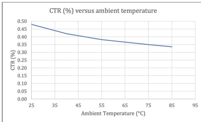
**Figure 3: Optocoupler Current Transfer Ratio vs. Ambient Temperature**
