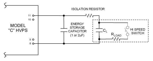
Note: The energy-storage capacitor and the isolation resistor control "pulse droop" during high-discharge-current conditions and average the peak current, thereby reducing the amount of time the HVPS is in peak current limit.
