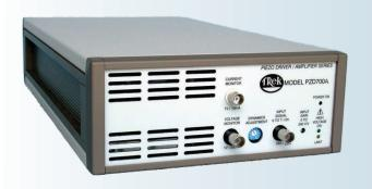
The Trek Model PZD700A is a high-voltage DC-stable piezo driver/amplifier designed to provide precise control of output voltages in bipolar or unipolar ranges which are customer specified within a range of available settings. The instrument achieves the accurate output responses and high slew rates demanded by reactive loads by utilizing a four-quadrant active output stage that sinks or sources current into reactive or resistive loads.
