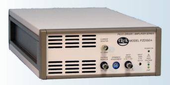
The Trek Model PZD350A is a high-voltage DC-stable piezo driver/amplifier designed to provide precise control of output voltages in bipolar or unipolar ranges that are customer specified within a range of available settings. It is configured as a noninverting amplifier with a variable DC gain. An inverting amplifier configuration is also available.
