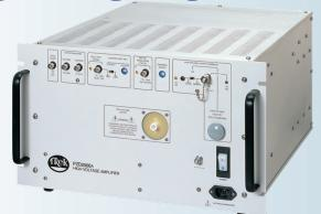
The Model PZD2000A is a wide bandwidth, high-voltage power amplifier used for precision high power applications. The amplifier incorporates an all-solid-state design for high reliability and low-noise operation. Its four-quadrant output stage sinks as well as sources load current throughout the output voltage range, thus achieving accurate output response and high slew rates, even into highly capacitive loads.
