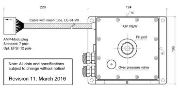
All plastic part components are flame retardant according to UL-94-V0, except viewing window. Glas viewing windows are available on request.
