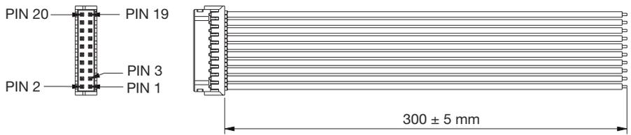
Order kit part number 73-788-001 for control connector interface with .3m wires attached
