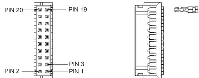
Order kit part number 73-788-002 for control connector interface with unloaded housing and 20 pins
