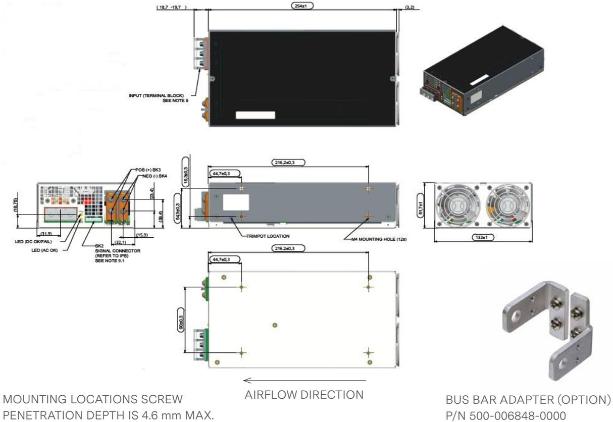
MOUNTING LOCATIONS SCREW PENETRATION DEPTH IS 4.6 mm MAX.
